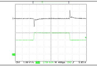
Figure 5: Output voltage response to step-change in load current (65 %-100 % -65 % of Iout(max);  $dI/dt = 0.1 A/\mu s$ . Load cap: 1  $\mu F$  ceramic cap. Ch 1: Vout, Ch 2: Iout (2.5 A/div).
