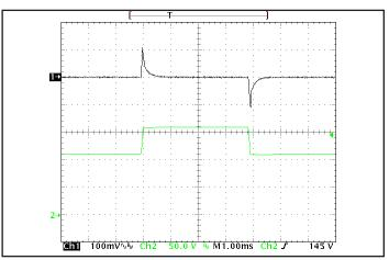
Figure 6: Output voltage response to step-change in input voltage (1000 V/ms), at Max. load current.Load cap: 15  $\mu$ F tantalum cap and 1  $\mu$ F ceramic cap. Ch 1: Vout, Ch 2: Vin.
