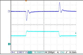
Figure 5: Output voltage response to step-change in load current (65 % -100 % -65 % of lout(max);  $dI/dt = 0.1 A/\mu s$ . Load cap: 1  $\mu F$  ceramic cap. Ch 1: Vout, Ch 2: lout (2 A/div).
