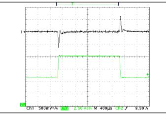
Figure 5: Output voltage response to step-change in load current (65 % -100% -65 % of Iout(max); dI/dt = 0.1 A/µs. Load cap: 15 µF tantalum cap and 1 µF ceramic cap. Ch 1: Vout, Ch 2: Iout (2.5 A/div).
