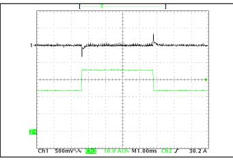
Figure 5: Output voltage response to step-change in load current (65 % -100 % -65 % of lout(max); dI/dt = 0.1 A/µs. Load cap: 15 µF tantalum cap and 1 µF ceramic cap. Ch 1: Vout, Ch 2: lout (10 A/div).
