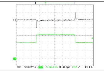
Figure 5: Output voltage response to step-change in load current (65 % -100% -65 % of lout(max); dI/dt = 0.1 A/ $\mu$ s. Load cap: 15  $\mu$ F tantalum cap and 1  $\mu$ F ceramic cap. Ch 1: Vout, Ch 2: lout (5 A/div).
