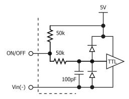
Figure B: Internal ON/OFF pin circuitry
