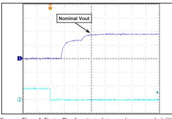
**Common Figure 1: Startup Waveform** (typical), input voltage pre-applied, ON/ OFF Pin on Ch 2.
