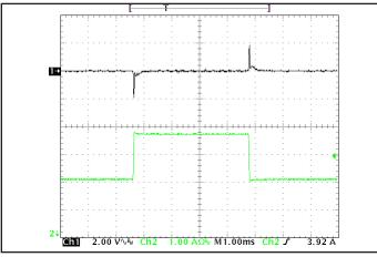
Figure 5: Output voltage response to step-change in load current (65 % -100 % -65 % of lout(max);  $dI/dt = 0.1 A/\mu s$ . Load cap: 1  $\mu$ F ceramic cap. Ch 1: Vout, Ch 2: lout (1 A/div).
