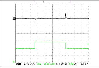
Figure 5: Output voltage response to step-change in load current (65 % -100 % -65 % of Iout(max); dI/dt = 0.1 A/µs. Load cap: 1 µF ceramic cap. Ch 1: Vout, Ch 2: Iout (2.5 A/div).
