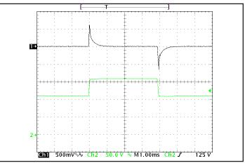
Figure 6: Output voltage response to step-change in input voltage (1000 V/ms), at Max. load current. Load cap: 1  $\mu$ F ceramic cap. Ch 1: Vout, Ch 2: Vin.
